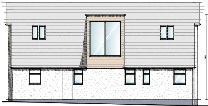
Proposed Rear Elevation Scale 1:50
